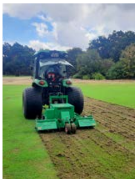
Photo 2: Scarifying with 'Graden' at St. Dionys Golf Club on 11 September 2024. (Photo: T. Fischer)
