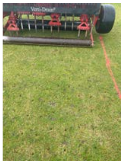
Photo 3: Deep aeration with Verti-Drain at Kalundborg Golf Club on 28 October 2024. (Photo: M. Truelsen)
